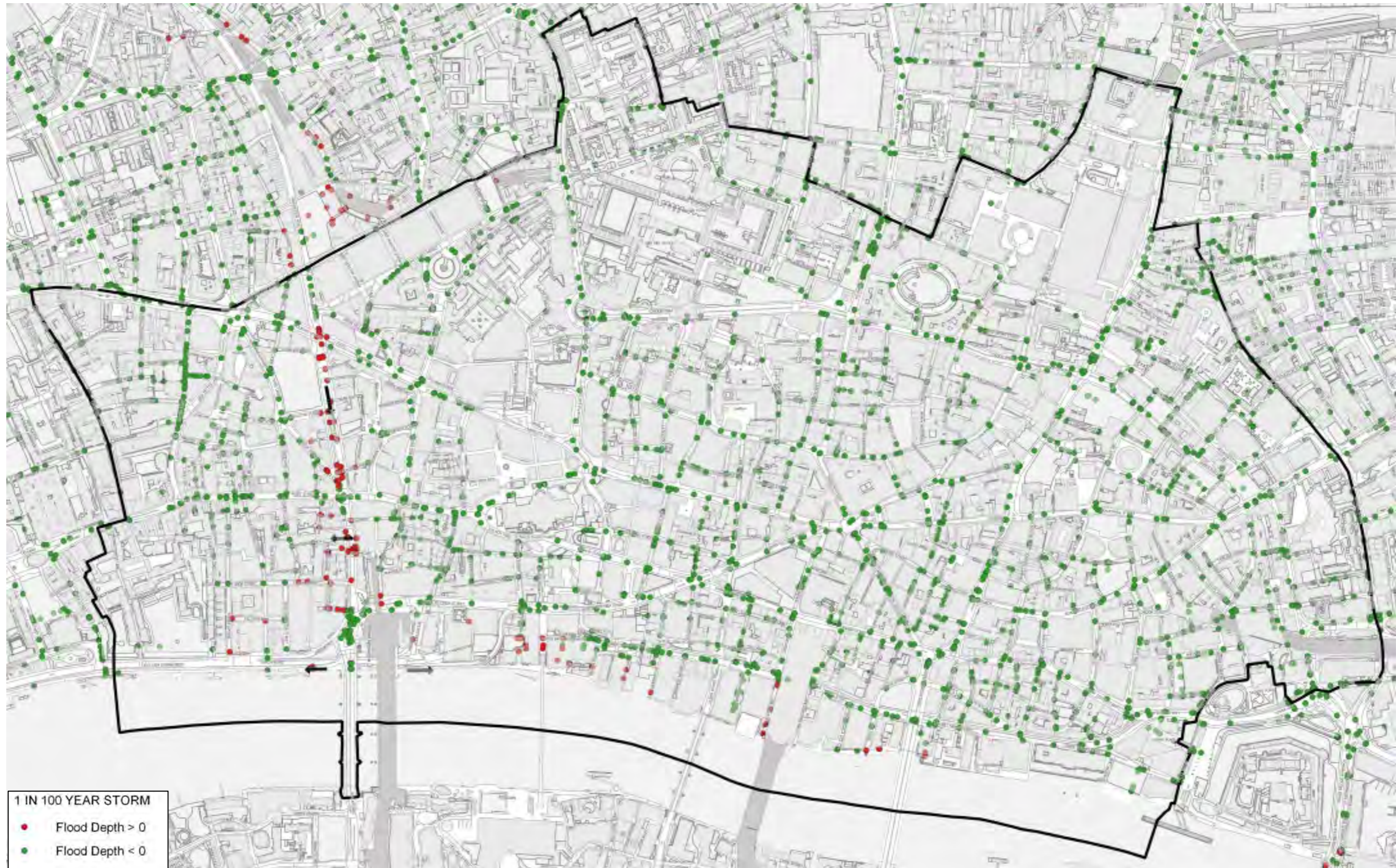
Figure C1 – Locations of Manholes Overflowing (2012 SFRA Model)
